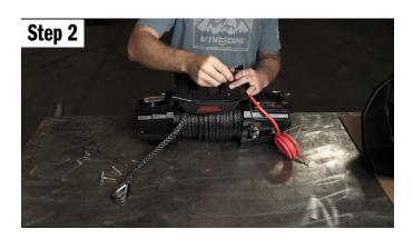
Start by removing the 4 allen bolts on the side of the winch that hold the top plate and controller in place. This will allow the winch to split apart, be careful to not pull it apart.
