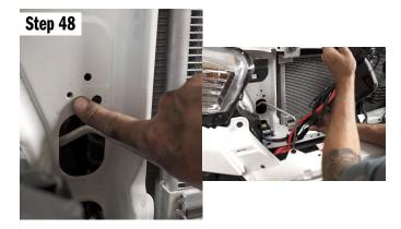
Place the mount in the truck. The top mount lines up with the threaded hole in the core support.
