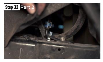
Next install the relocation bracket. Place a washer on the 5/16 bolt and push it through the power steering line bracket, then through the hole of the provided bracket. Then put the factory bolt back into the slot on the bracket. Leave loose for now.
