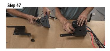
First we need to install the controller to the mount. This mount is designed specifically for the Smittybilt and Warn winches we list. It may work for others. Line up the mounting holes and ensure the wires are pointed the correct direction, then install the bolts included with your winch.
