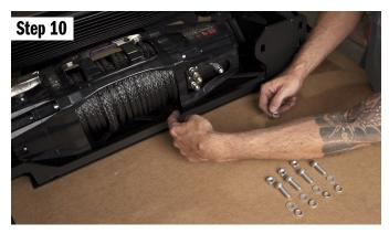
Bolt the winch to the bumper using the hardware provided with the winch. For the Smitty and Warn winches, you will slide the square nuts into the winch body.
