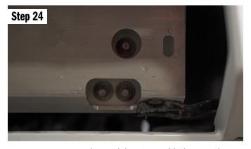
Now we can remove the crash bar. Start with the nuts that hold the long bar in place. There are 3 on each side. Remove the nuts. Then there are 3 more nuts on each side that hold the bar to the frame. Remove those nuts as well.
