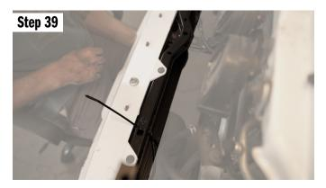
Put the LED in place behind the lower grill, and with your zip ties or string, wrap them around the factory grill support and tighten them so the LED stays up and in position. With the LED up and out of the way, we can now install the bumper.
