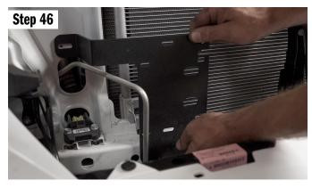
With the bumper installed, we can now install the winch controller and mount. In this image we see the placement of the mount. The wires to the winch will need to exit the left side of the mount to reach the winch.
