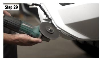
Using a cutoff wheel, dremil, sharp knife or other cutting tool, trim away the plastic.
