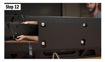
Push the bolts through the bumper and into the winch. Tighten everything down in place.
