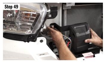
Take your M6 bolt and install a lock washer and flat washer, then push the bolt through the mount and thread into the core support.v
