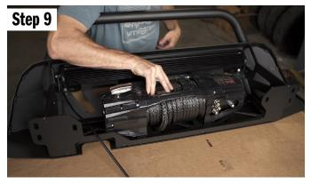
Next we will prep the bumper. Grab your winch and put it in place. If the winch line is already installed, ensure it is pushed through the fairlead before tightening in place.
