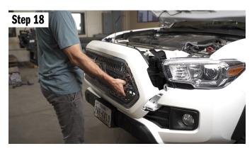
With the hardware removed, pull the grill forward and remove.
