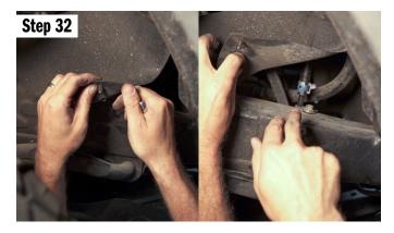
There is also one additional bolt that holds the power steering line in place. Remove the bolts to the line can move freely. You can access this on the passenger side right behind the front mud guard.
