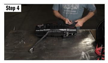
Re-install the top plate back on the winch.
