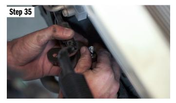
Install the washer and nut, do this for both positions. Then like the line, install the factory bolt through the slot in the relocation bracket. Push the cooler towards the radiator, then tighten the cooler in place. With the cooler in place, now tighten the line bracket in place.
