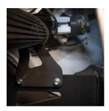
Optional - If you have the hidden upper LED, cut the zip ties or string. Then manouver the brackets in place. They both go on the inside of the vertical bumper brackets. With them inside, put a washer on a 1/4 bolt, push the bolt through the bumper, then the LED mount. Then put on a washer and nut. Do this for all 4 positions. With the mounts in place, push the LED forward. Tighten the LED to the mounts, then the mounts to the bumper.
