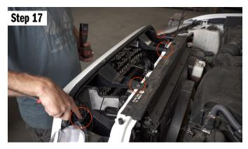
Truck Prep - Now we can prep your truck. Start by removing the grill. There are two bolts on top, there are also two plastic clips on top. If you have the Safety Sense radar, don't forget to unplug that and remove the ware clip from the grill.
