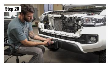
If you have a front license plate, remove it. The screws for the plate mount are behind the plate itself, remove the mount as well.
