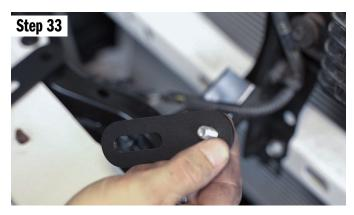
We will now do this for the cooler itself. Follow the same step of putting the bolt through the bracket and into the bracket on the cooler.
