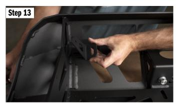
Optional - LED Mounts inside the bumper. If you are installing an LED in the bumper, we first need to install the mounts. They are adjustable to fit multiple lights. Orient the mount so that it is pointing forward, and the L-Tab is pointing inward.
