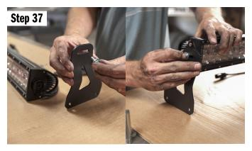
Optional - If you also purchased the top / hidden LED mount, we need to get it prepped and in place before we install the bumper. If not, you will not be able to get the LED in place. Start by bolting the mount to the LED. Making sure the mount is pointing forward towards the front of the LED
