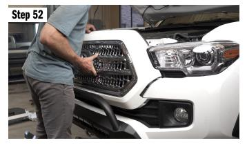
Lastly, re-install the grill. Push it into place, then put the two plastic clips and two bolts in place. If you have safety sense, plug it back in.
