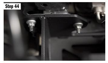
Now tighten all the nuts to the frame, 3 on each side.
