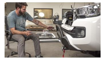
Now check the bumper for straightness. The holes are slotted for up and down adjustment. Get it in the position you desire.
