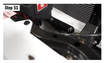
Then bellow are two bolt opportunities. You only need to install one. put a washer on your 5/16 bolt, push through the mount and core support. Then install the washer and lock
