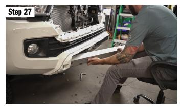
Then with the extra space, you can slide the crash bar to one side, pop it out, then fish the rest out and remove.
