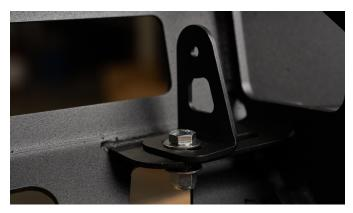
Grab a 3/8 bolt, install a washer, push through the bumper and mount, and install another washer and lock nut. Leave hand tight.
