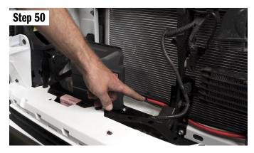
Now that the winch controller is installed, you will need to run the wires. Following the instructions for Smittybilt, install the wires from the winch controller to the winch in the order called out. For Warn, the wires and studs are color coded. Connect green to green, blue to blue, yellow to yellow. For both, you will also have a positive and negative that go to your vehicle battery. Route the wires and install. Test winch functionality after wiring.
