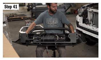
Now we can install the bumper. We highly recommend you use the help of a friend or two. Get the bumper into position and push it into the truck.
