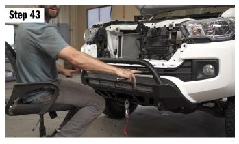
Now put on the remaining nuts. Start with the nut that is on the inside of the frame. Tighten them up allowing the bumper to pull up and into position on the truck. Tighten inner bolt on each side until it is snug.
