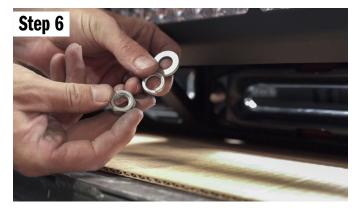
We recommend using the hardware that comes with the winch and fairlead, in most cases it is a bolt, washer and lock washer or nut.
