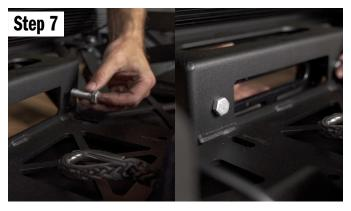
IMPORTANT NOTE - The winch is tight to the bumper. Depending on your hardware and fairlead, you may need to install the bolt from the back, to keep this clear, and move the taller nut and washers to the front.
