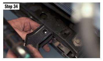
Put the relocation bracket on the bottom and push the bolt up though the mount,
