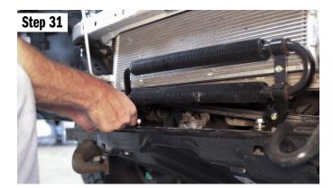
The next step is to relocate the power steering cooler rearward. Start by removing the two bolts in the front that attach it to the frame.
