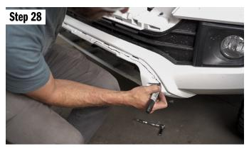
Now it is time to cut. You will see a lip that followed the old trim part in place. We want to cut the center out so that there is a 1/2 to 5/8 lip remaining. Mark with a sharpie. Also you do not need to cut the center of the top, go only to the 2nd clip hole as shown above.
