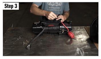
With the top plate removed, flip it over and take out the 4 smaller allen bolts that hold the controller to the top plate. Also disconnect the wires from the back of the winch, leave them connected to the controller.
