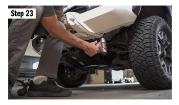
Now we will remove 4 bolts that hold the aluminum crash bar to the bumper. There are two in the center, and one on the passenger and drivers side.
