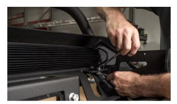
Tighten the mount to the bumper. Your bumper is now ready for install.
