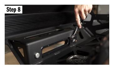
Tighten the fairlead hardware in place.
