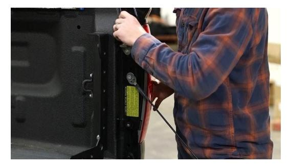
For this tightening sequence, start with the vertical side and finish with the bottom. First, tighten the 2 vertical side bed support bolts, as well as the tiedown hook. Finish with the 2 bottom side bed support bolts, as well as the bed bolt.
