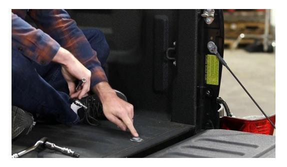
The first is the tiedown-hook, and the second is the bed bolt. For the tiedown-hook, grab your ratchet with a T40 socket and remove each screw. As for the bed bolt, that will require a Torx T55.
