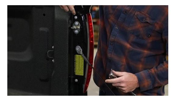
First, you will need to remove the taillight using a ratchet and a T30 socket. On your truck bed, directly behind the taillight, you will notice 2 bolts, 1 at the top, and one at the bottom - remove them.
