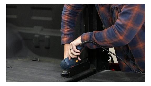
Now it's time to install the bed support. Start by lining it up with the holes left by the previously removed tiedown-hook and bed bolt. Then, loosely screw them back in place. With everything lined-up and in place, you can mark the hole center using the drill with a 3/8" drill bit.
