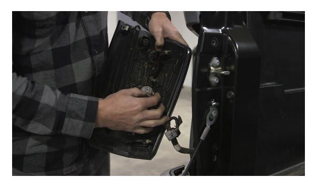
There are 3 wires connected to the tail light, simply squeeze the tabs and pull them apart.
