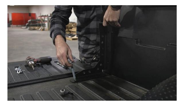
To install the bed supports, place it into position, and replace the bed bolt and tie-down bolt, hand tightening them for now.
