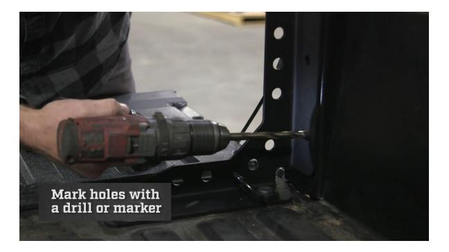
Before marking the holes, make sure the bed support is pressed firmly against the side of the bed. Then, grab a sharpie (or use a drill) to mark the centers.
