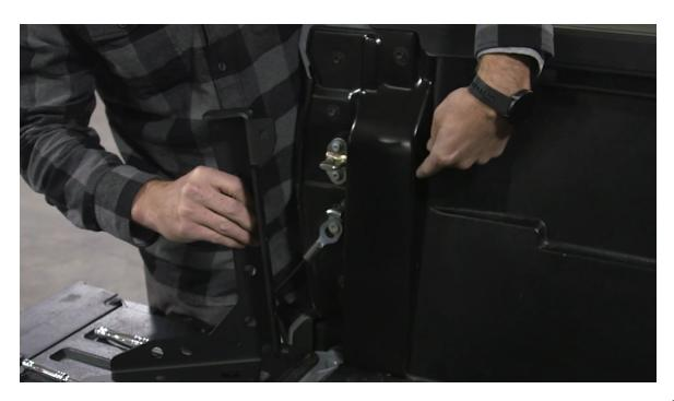
With the hardware removed, you can now position the bed supports into place. Be sure to line up the tab on the top of the bed support with the backside of the mount (shown above). Once it's there, insert the bed bolt and tie-down bolt and hand tighten them.
