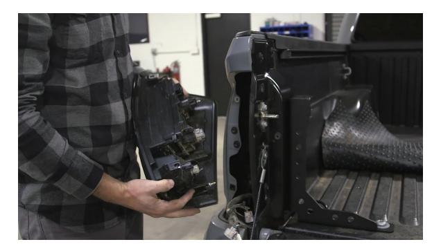
To reinstall the tail light, you'll first need to connect each of the 3 plugs. Each is different, so it's not possible to plug them into the wrong spot. Then, place your tail light back into position, and push it against the bed.
