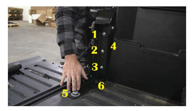
You're nearly done! The last thing you need to do is tighten everything down. However, it's very important that you follow the correct tightening sequence (shown above). The bed bolt and tie-down bolt should be tightened last.
