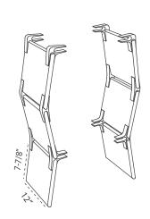
1 Assemble vertical groups using only B boards and the illustrated connectors.
