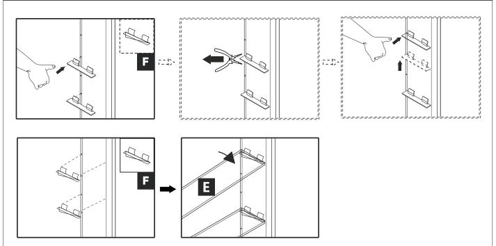
1.Insert clear snap in shelf clips (F) into holes on the sides of the cabinet cabinet.
