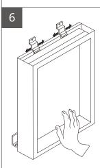
Make sure top brackets are locked in the grooves.
