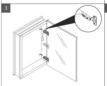
While supporting the door release(the lever under the hinge arm), slide the door off the frame.
