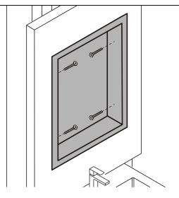
Affix using hardware screws into the studs.
