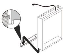
With assistance, to rest the cabinet on the mounting bracket and hold in place.
