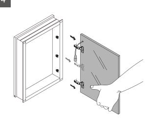
Take off the door(s) carefully and lay it down on a safe area.
