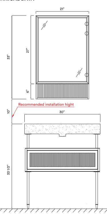
**ATTENTION!** Dimensions may vary by up to 3/8". It is highly recommended to pull all dimensions of actual model for installation and measuring purposes.
