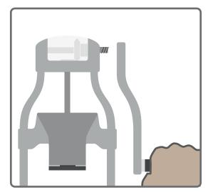
2. SELECT THE GRIND WITH THE HANDLE AT IT'S LOWEST POINT ROTATE THE WHEEL TO YOUR REQUIRED SETTING
