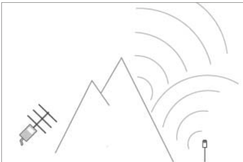
The mountain deflects the signal depriving the receiver.
