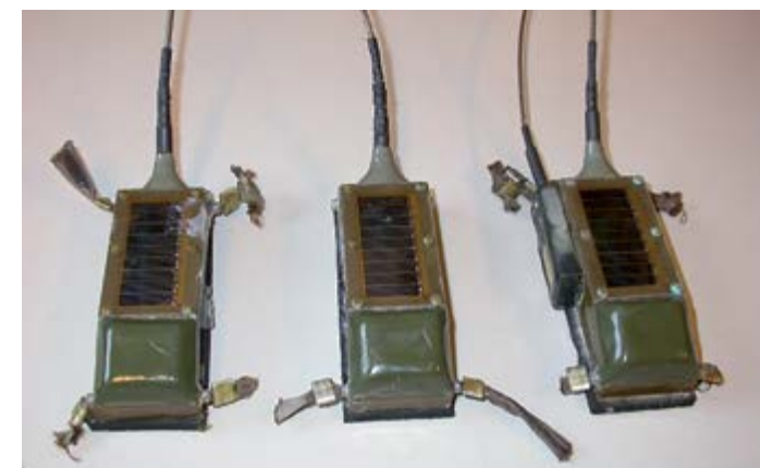
Figure 20. Three GPS transmitters from young Golden Eagles found in the field in northern Sweden where human persecution was implicated. The teflon ribbons were cut off with a sharp object. The transmitter to the left was found together with remains of the bird on a municipal sewage-dump. Photo: Torgeir Nygård.
