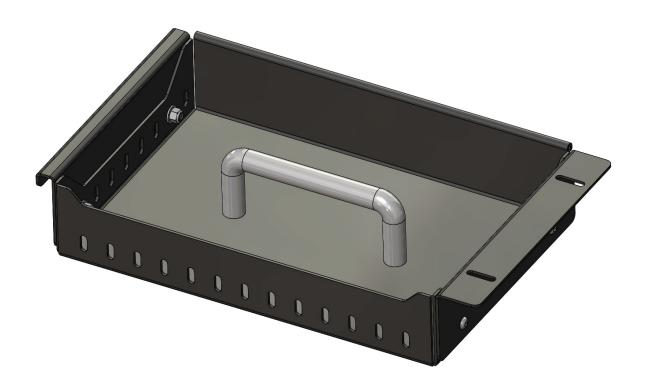
4. Using (2X) 1/4-20 X 5/8 Button Head Bolts, (2X) 1/4 Flat Washers, (2X) 1/4-20 Nylon Lock Nuts install the Hanger as shown below. The head of the bolt should be on the top of the Tray placing the Lock Nuts on the bottom.
