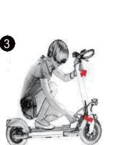
Move the handlebar bar back and forth to check that it does not move and is fixed. Check the brake drive.
