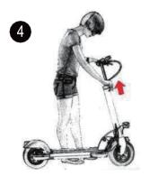
Turn the handlebar fixing lever and raise the bar to the desired position. Once raised, tighten the handle.
