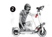
Raise the lever to fix the folding handle while firmly holding the folding bar.
