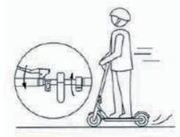
4. Release the accelerator finger to decelerate and press the brake if you wish to brake.
