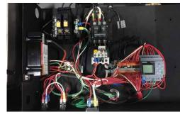
**PROGRAMMABLE SMART CONTROL** now standard for all VGH machines allows auto start/stop and time delay shutdown features without changing any hardware. It also provides complete control of the equipment run time.
