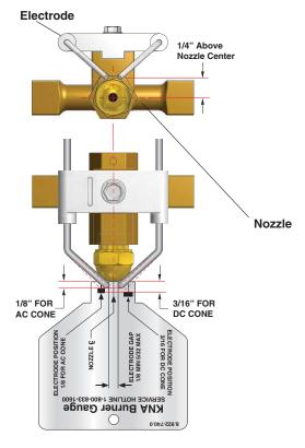
Periodically Check Wiring Connections. If Necessary To Adjust Electrodes, Use Diagram.
