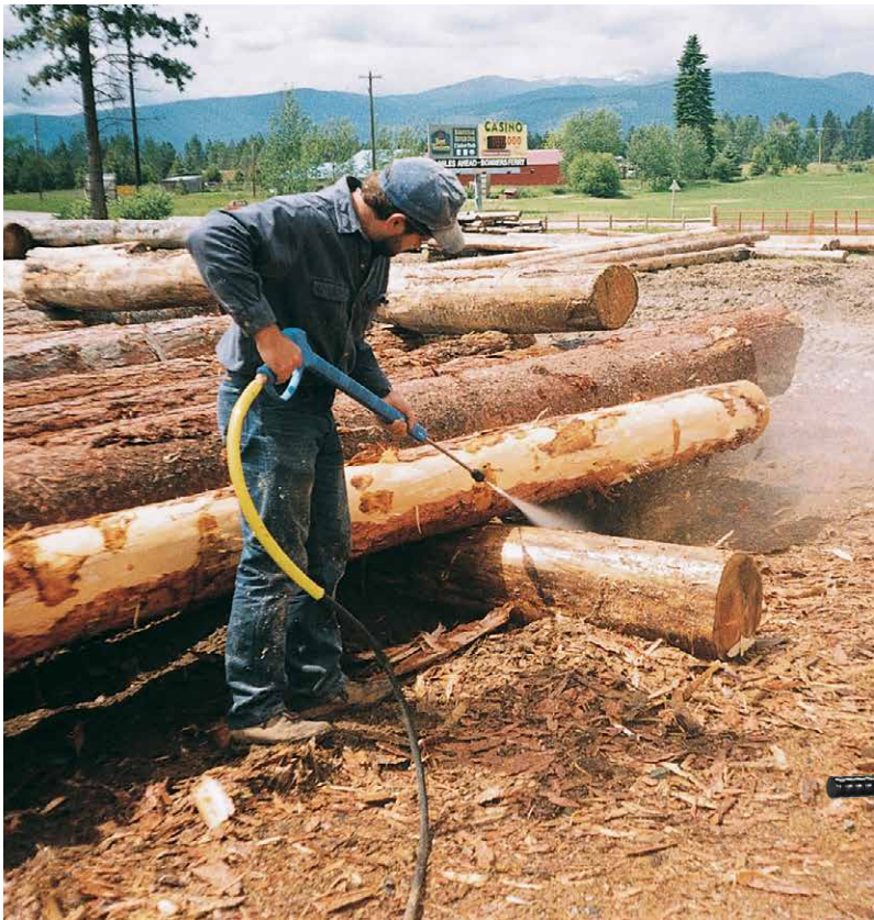
Stripping bark from logs is only one of the many applications for the MP high-pressure washers with cleaning power of up to 5000 PSI.
