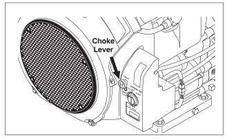
**STEP 5:** Pull the choke lever out to the "Choke" position (on a warm engine, leave the choke lever in, in the run position). Push the choke lever to the "Closed" position. To restart a warm engine, leave the choke lever in the "Open" position.
