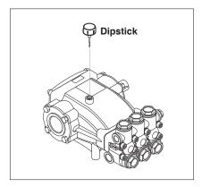
**STEP 4:** Remove shipping cap and install oil dipstick. Check pump oil level by using dipstick or observe oil level in oil window (if equipped). Use 20/40W non detergent oil.
