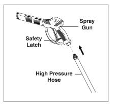
**STEP 1:** Attach the high pressure hose to the spray gun using teflon tape on hose threads.
