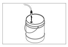
STEP 1: Remove detergent suction tube from container and insert into one gallon of fresh water. For low pressure connect the black detergent nozzle. Pull trigger on spray gun and siphon water for one minute.
