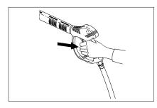
STEP 3: Press trigger to release water pressure.
