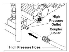
**STEP 3:** Connect the high pressure hose to the high pressure outlet. Push coupler collar forward until secure.
