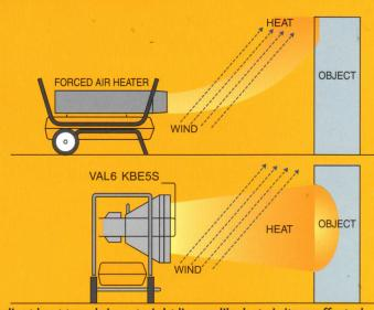
Radiant heat travels in a straight line, unlike hot air, its unaffected by wind or cold ambient air. Since infrared heat can penetrate into the object, the targeted surface and object are warmed and/dried in a uniquely different way from any convectional heater which utilizes heated air.
