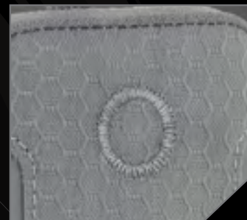
Circular Reinforcement Bartacks
