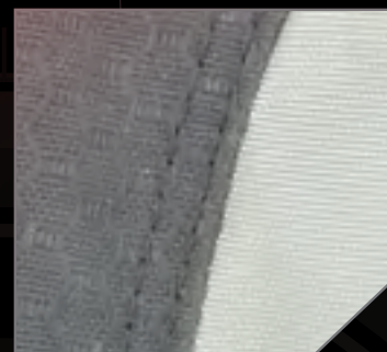
Dual Nylon Fabric Construction 420D Plain Weave/ 500D Hex Ripstop
