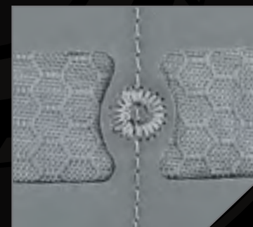
Circular Reinforcement Bartacks
