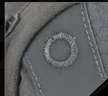
Circular Reinforcement Bartacks
