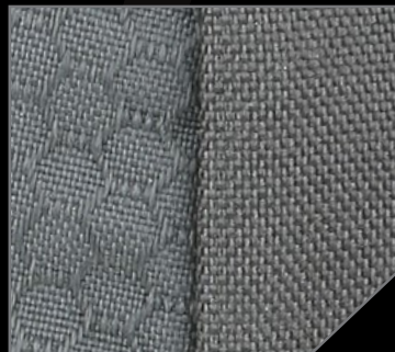
Dual Nylon Fabric Construction 500D Hex Ripstop / 1000D Plain Weave
