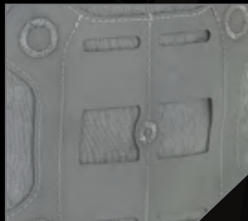
ATachment Lattice System - ATLAS™ Cut from 840D Nylon-TPU Composite
