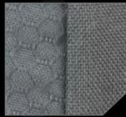
Dual Nylon Fabric Construction ATtachment LAttice System - ATLAS™ Anti-Counterfeit Logo 500D Hex Ripstop / 1000D Plain Weave
