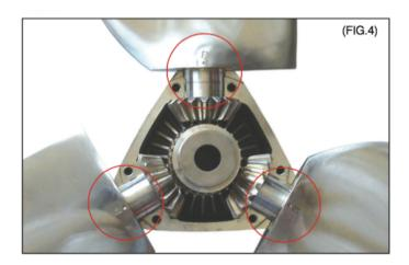
NOTE: the propeller in Figure 4 is set up for right hand rotation. If it was for left hand rotation you would see the L stamps.
