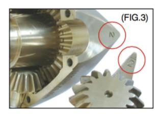
With the hub in the correct location in the forward body (as above) the blades can then be inserted taking care to put them in the matching numbered journals and in the correct position (with the blade datum in the 12 o'clock/uppermost position as in FIG.4).
