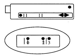
Hold unit with second finger and thumb on both hands and slide scale with left index finger. Push power button with right index finger. Slide scale until laser light line #2 is on the 0 of the scale. Take reading at laser light line #3.
