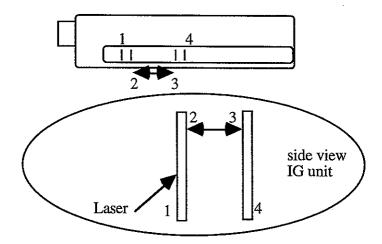
A dual pane will show 4 reflections, the laser is mounted at  $45^{\circ}$  to the glass surface so the distance between the lines will be 2 times the air space. The scale is actually 2:1 but reads direct. (4 or  $1/2^{"}$  reading on scale is 1 inch of actual distance).
