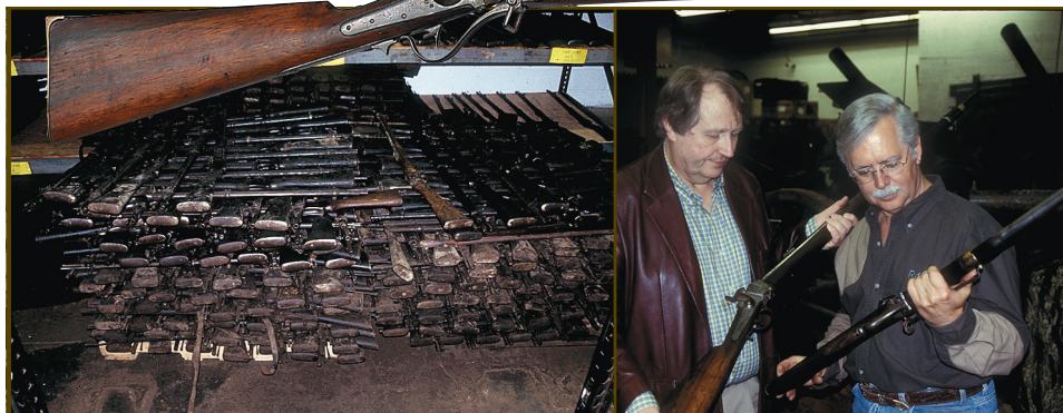
The author (r.) and IMA President Christian Cranmer (l.) inspect a pair of the mysterious Nepalese Sharps rifles. The Sharps rifles (above) featured 40" long barrels and were apparently intended to be fitted with socket bayonets. The Sharps carbines were all brass-mounted and fitted with 20" barrels and ladder-style rear sights. Both had Lawrence pellet primers and unique sling swivels (above l.) that replaced the normal hinge pins.
