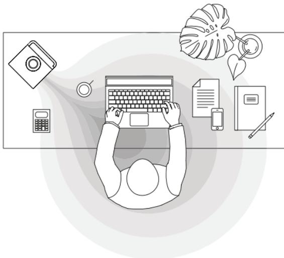
The air cooler creates a local comfort zone. To be in the center of that zone place the device within a meter (3 ft.) away from you, with its front grill facing you. To keep the device out of your way, place it slightly aside. This way you will always have room for a laptop or a book.
