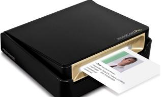
Hardware Specifications: Dimension (L x W x H): 107 x 28 x 100 mm) Weight: 168g Resolution: 600 dpi Interface: USB Windows 7 / Mac OS X 10.11 or later
