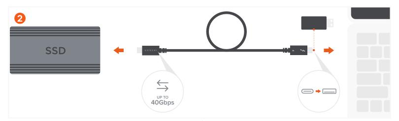
Connect Thunderbolt cable to your USB-C or Thunderbolt 3/4 host devices for fast data transfer speeds up to 40Gbps. Backwards compatible with Thunderbolt 3, USB 3.2, USB 3.1, USB 3.0, USB 2.0. USB-C to USB-A adapter not included.
