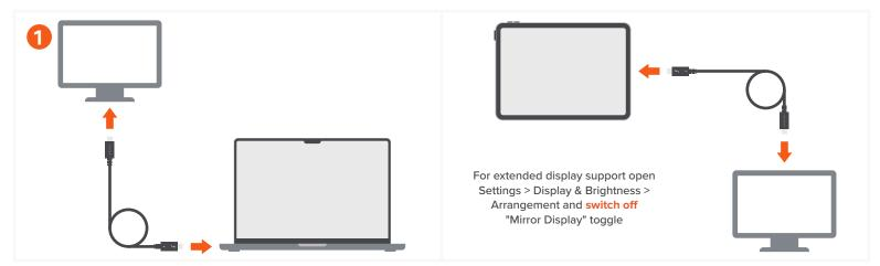
Connect Thunderbolt 4 Pro Cable to USB-C or Thunderbolt external monitor. Supports single display 8K@60Hz or 4K@120Hz, and dual display 4K@60Hz. For dual display output must use two Thunderbolt cables.
