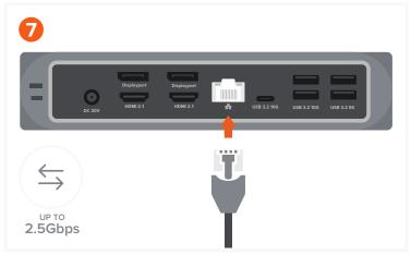
Connect an RJ45 Ethernet cable to the dock's Gigabit Ethernet port.
