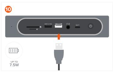
Use the USB-A 2.0 port for charging a USB device – up to 7.5W.
