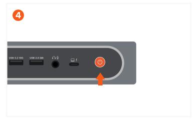
After connecting the dock, press the power button on the front of the dock to turn it on.
