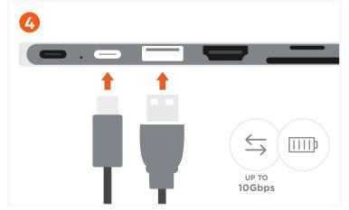
Use the USB-C and USB-A ports for fast data transfer speeds – up to 10Gbps
