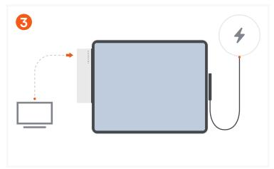
When using the USB4 port for video output, it is recommended to use the proprietary charger to keep the Surface Pro 9 charged unless your connected monitor supports charging.
