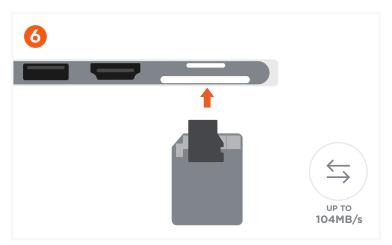
Insert microSD or SD cards into the card reader slots. UHS-I speeds - up to 104MB/s. Supports synchronous use.
