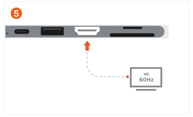
Use the HDMI port to output up to 4K / 60Hz with an external monitor.
