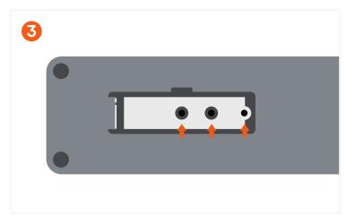
Remove the film from both sides of the included thermal pad and align the holes on the thermal pad with the screw openings.
