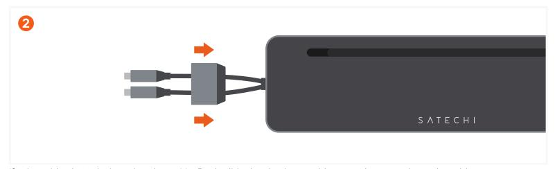
If using with a host device other than a MacBook, slide the aluminum cable cover down to release the cables. Both cables must be connected in order for full functionality
