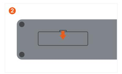
To install the SSD, press and lift the latch on the SSD cover.
