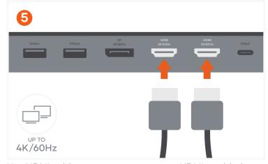
Use HDMI cables to connect up to two HDMI-enabled monitors.
