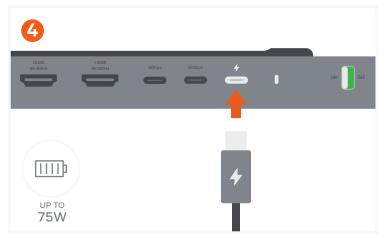
Use the USB-C PD port to charge your device up to 75W. ~15W is used for the docks operation USB-C charging port does not support video output or data transfer
