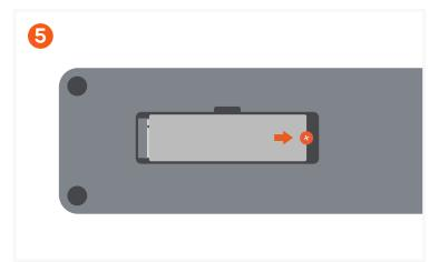
Use the included screw and screwdriver to secure the SSD into place.
