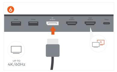
Use DisplayPort cable to connect to a DisplayPort-enabled monitor.
