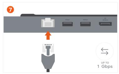
Connect an RJ45 Ethernet cable to the dock's Gigabit Ethernet port.
