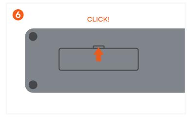
Reinstall the SSD cover. Insert at an angle and press down until it clicks.
