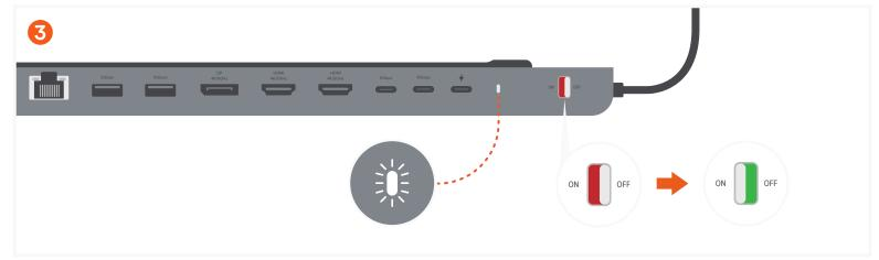
Slide the power switch to the left from red to green in order to turn on the Dock. White LED will turn on signifying the dock is on
