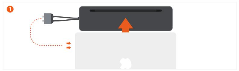
Connect the dual cable connectors to the dual USB-C ports on your host device. Both cables must be connected in order for full functionality
