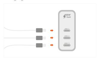
3 Connect and charge up to three USB-C devices at the same time.
