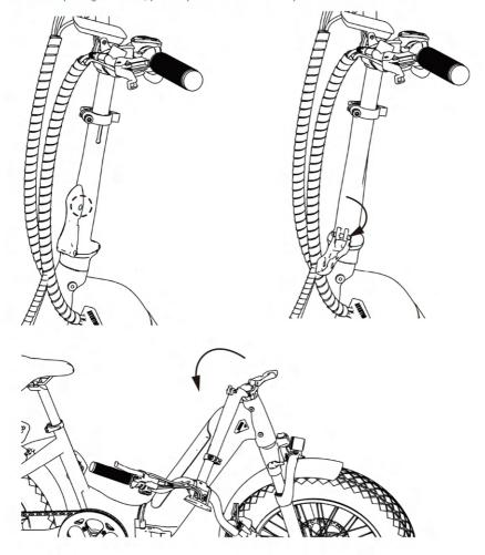
4. Holding the latch lock up, use your other hand to open the latch by pulling it away from the frame, folding the rear wheel/section towards the other wheel and use the stand under the frame as needed.
