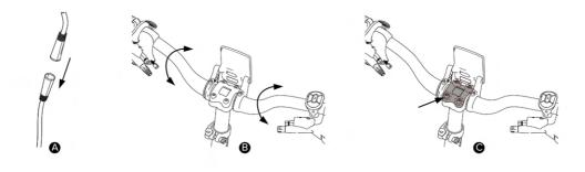
**Step 4.** Use a 3mm hex key to loosen display screws. Then install display onto handlebar using 3mm hex key and tighten screws.
