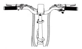
**Step 5.** Release the clamp under the handlebar, pull the handlebar up or push it down to adjust height as your desired, then close the clamp to secure handlebar in place.
