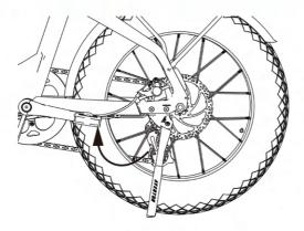
Step 8. Put on the motor protection guard on both sides of back wheel. Install motor protection guard on both sides of back wheel.
