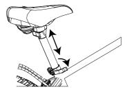
Step 12: Adjusting the seat position and angle
