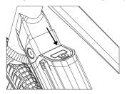
"Press and hold the "M" button on the display unit to turn on the display."
