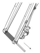
B.Remove the plastic insert card from the front brake caliper.
