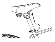
If needed, use the thumb nut to add tension to the clamp so there is some resistance when the lever is in line with the clamp bolt, but do not overtighten. Close the quick release lever to secure the seatpost and check that it cannot move. See the Adjusting the Seat section of this manual for more details.
