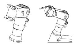
**Step 6:** Place the handlebar on the stem correctly. Center the handlebar and screw in the four stem faceplate bolts evenly, however do not tighten all the way down for further adjustment.
