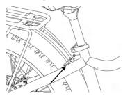
C. Remove the screws on the bracket. Install the bracket in between the rear stays, and fix it in place with attached M5 washers and screws.
