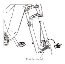
D. Use 15mm open wrench to tighten front axle nut, recommended torque value at 25-30Nm.
