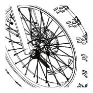
**Caution:** Never touch the brake rotor, especially when the wheel and/or bike is in motion, or serious injury could occur. Hand oils can cause squeaking and decrease brake performance
