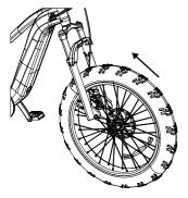
B. Remove fork protective cover and take out plastic insert from front wheel brake caliper.
