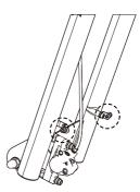
B.Align front fender to the screw holes, use 4mm hex key to tighten front fork screws. (3 pcs)
