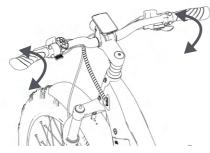
B. Stand in front of the bike and clamp front wheel between both legs, verify the handle bars are straight and in line with the front wheel. Make sure the pinch bolts are tight and you can not turn the stem freely from the front wheel.
