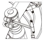
D. Adjust display to the desired position, tighten the screws with 2mm hex key.
