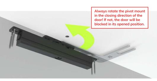
(4) Use the drill tool to rotate the pivot mount in place. Repeat for the bottom pivot mount.
