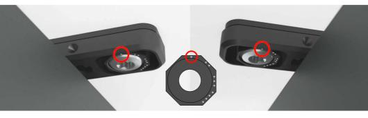
(5) Install the octagonal inserts at 'position 1' in the top mount, then insert screws but do not fully tighten yet. Repeat for the bottom mount.
