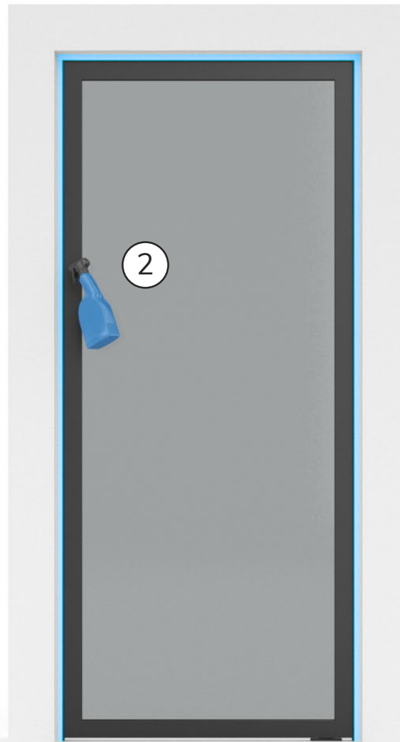
Moisturize sealing product and framework with water and soap.
