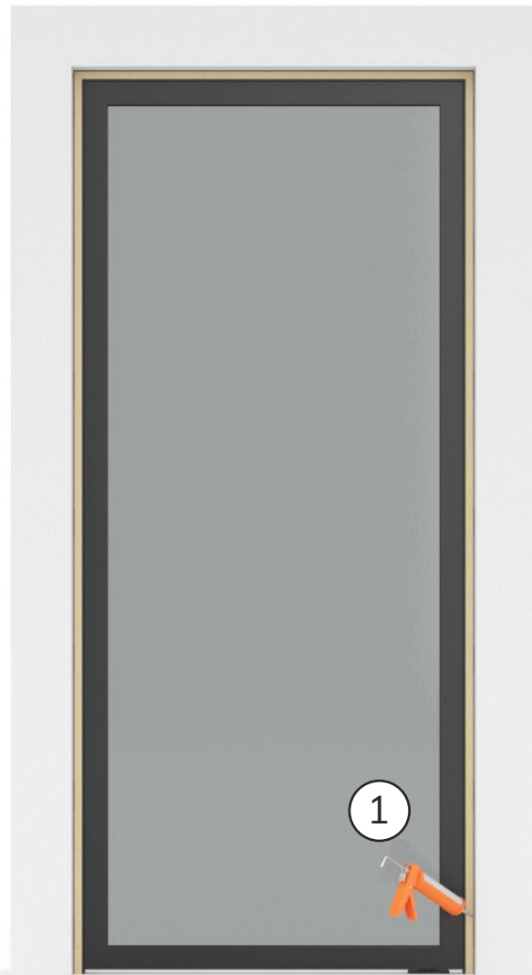
Finish the joint with a paintable sealing product.
