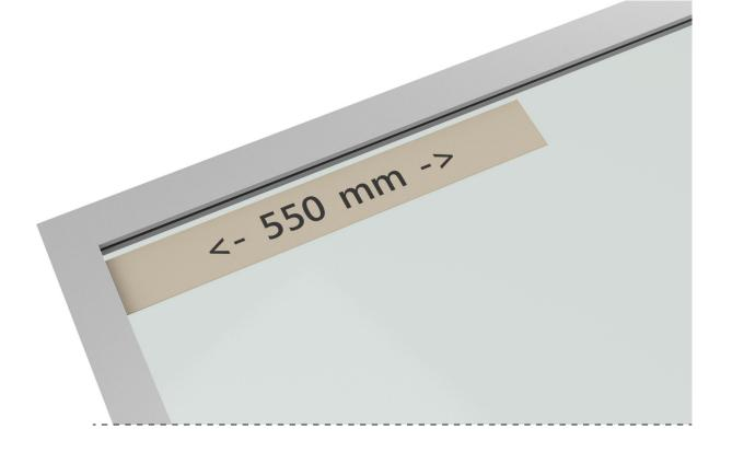
Place the correct length guide in the bottom left corner.
