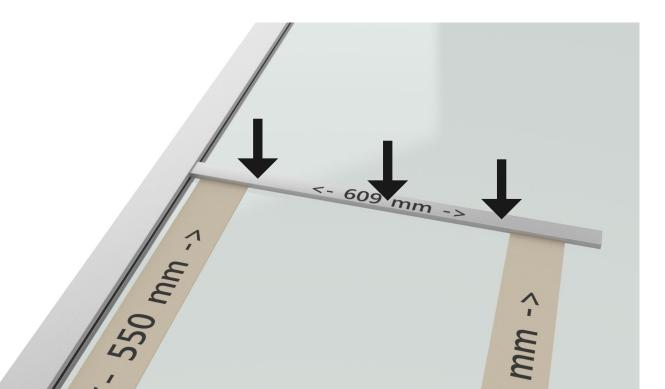
Use the length guides to position the grid profile onto the glass.
