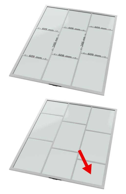
Repeat steps for all remaining grid profiles, using the correct length guides and grid profiles (according to your design).
