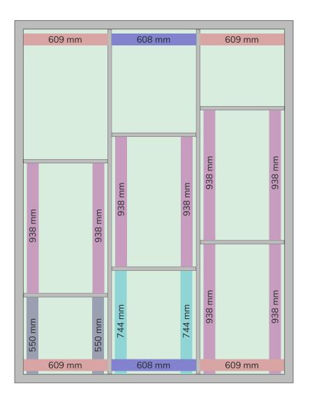
Example measurements in this manual use 30 mm wide grid profiles on a 5730 door!
