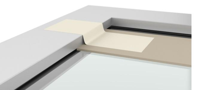
Use masking tape to keep the guide in place.
