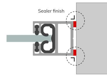
Moisturize the sealing product and framework with water and soap, to finish the sealing joint under a straight angle with a rectangle tool / spatula.
