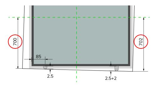
To level the panel, the right side should be raised from 2.5 to 4.5 mm.
