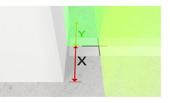
Position the other laser plane exactly on the desired center location (In this example, X=Y)
