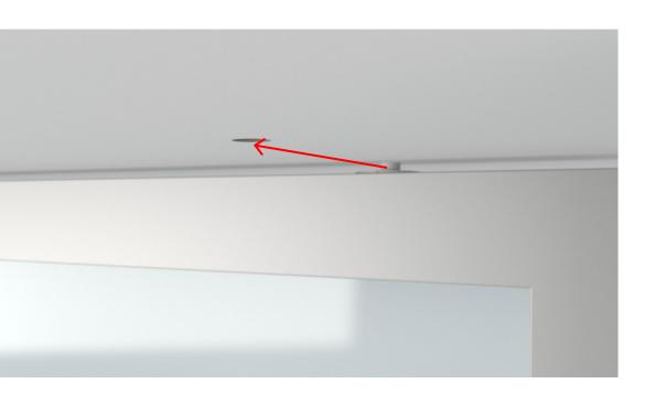
Carefully rotate the panel in place, untill the top positioning caps extend in the ceiling holes.
