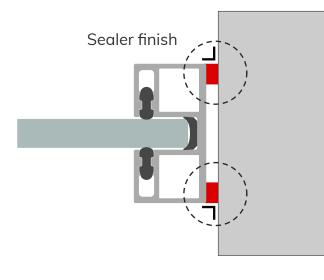
Moisturize the sealing product and framework with water and soap, to finish the sealing joint under a straight angle with a rectangle tool / spatula.
