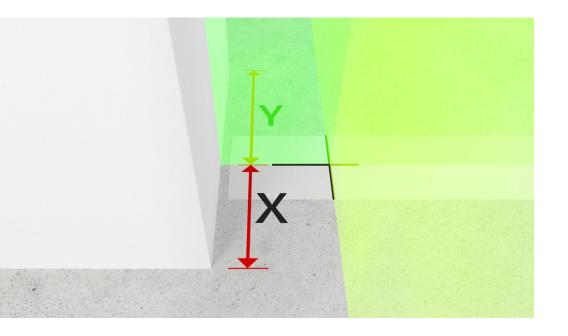
Position the other laser plane exactly 12 mm off the desired panel center location.
