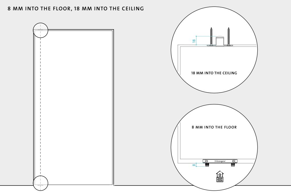
The top pivot and bottom pivot hinge system components are fully-mortised in the pivot door. Only small floor and ceiling plates are visible. The floor plate fasteners only need to be mortised 8 mm into the floor, which means every FritsJurgens system can also be utilized in combination with radiant floor heating.
