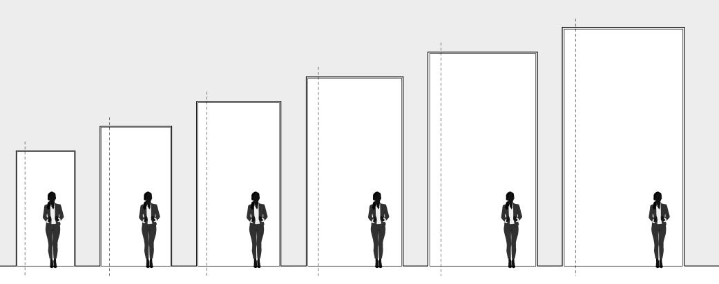
Each FritsJurgens pivot system is suitable for light and heavy doors. System M+ comes in models tuned for doors from 20 up to 500 kg. System M is suitable for door between 20 and 210 kg. System One also supports doors up to 500 kg, while System 3 supports doors from 40 to 350 kg. The possibilities for the design of the door are endless and the movement is smooth and fluent.
