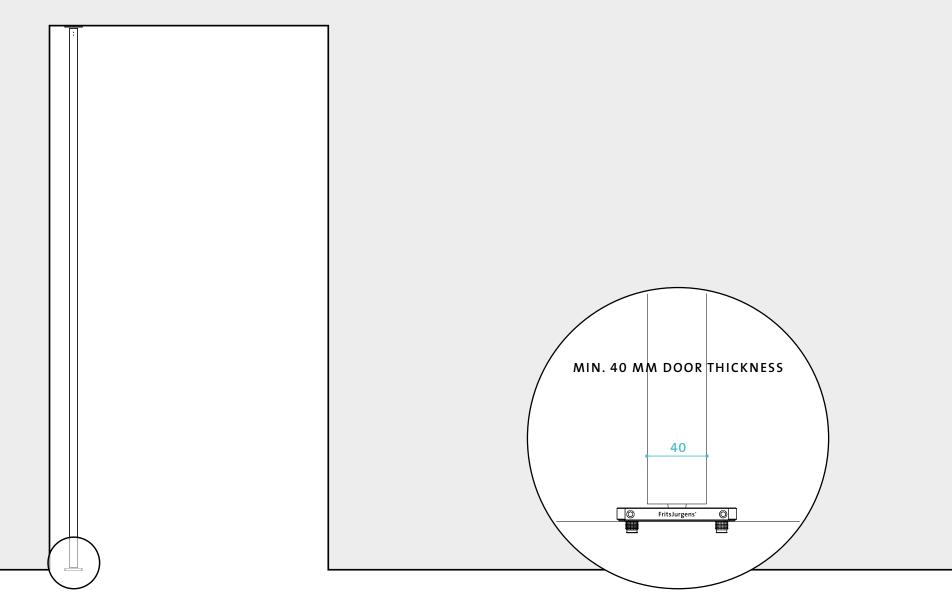
Since the FritsJurgens pivot hinges have a thickness of 32 mm (or 42 mm) they can be used in doors with a minimum thickness of 40 mm. This makes FritsJurgens systems suitable for doors of virtually any size and material, giving designers the freedom to design the ultimate pivot door.
