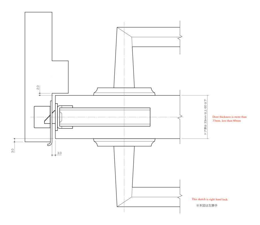
$\begin{array}{c} & 2015.03 \\ \text{Mortise Lock Case} & S=1/1 \end{array}$
