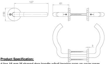
d line 16 mm M shaped door handle w/ball bearing snap on cover roses cc38 mm, 8x8 mm spindle, for doors 33-44 mm, AISI 316
