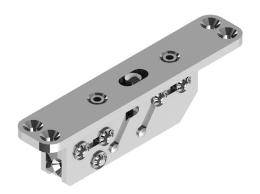
The top pivot is integrated into the top of the door and uses a so-called pin/hole connection. The pin is fixed to the top pivot and drops into the hole in the ceiling plate when this is turned.
