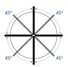
Below each 45° angle, the door automatically moves from both directions to the hold position.
