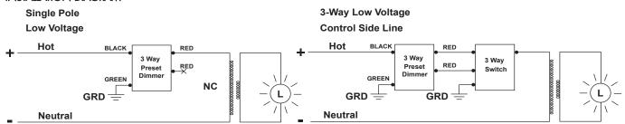
**NOTE** It is normal for the dimmer to feel warm during operation. Use a separate neutral wire for each phase of a multiphase system containing a dimmer, and for high power single phase applications where flickering is present.
